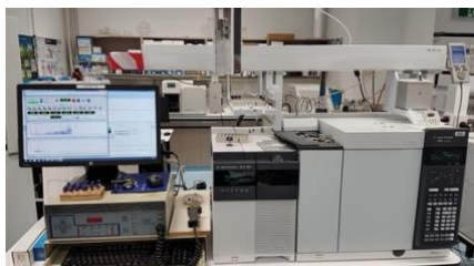
Photo: GCMS system used to characterise organic fractions during thermophilic composting
