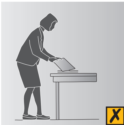
Figure 4.8 Incorrect standing-height bench
